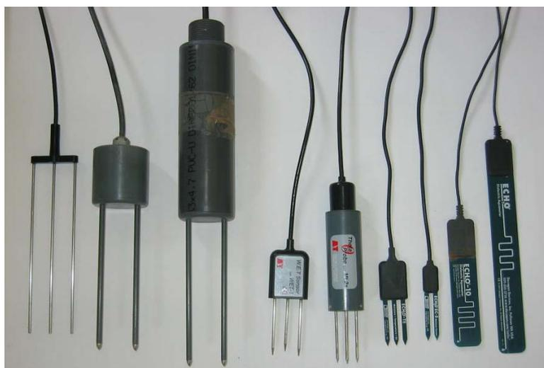
**Figure 1.** EM sensors investigated. From left to right: 3-rods Trase probe, TRIME-P2, TRIME-EZ, WET Sensor, ML2x, ECHO-TE, EC-5, EC-10, and EC-20.
